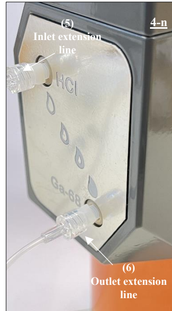
Fig. 23 Connecting the Inlet end (female LUER end) of the outlet extension line (6) to the Ga-68 port via the adapter.
