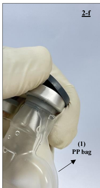
Fig. 14 Removing the cap from the PP bag containing the 220 ml sterile 0.1 mol/L hydrochloric acid solution (1).
