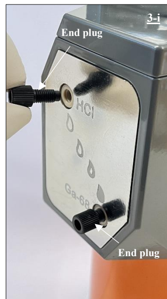
Fig. 18 End plug covering the HCl port of the radionuclide generator, prior to removal.
