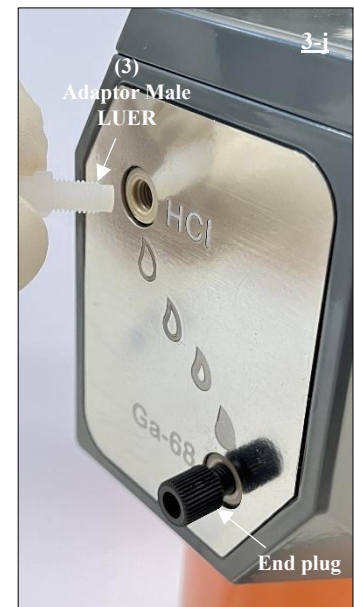
Fig. 19 Attaching the male LUER adaptor (3) to the HCl port of the radionuclide generator.
